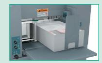
for a longer period of time without constant reloading. To ensure the accuracy of each booklet, the DFS-3500 uses a double feed detection sensor to stop the machine when it detects two or more sheets have been fed.
