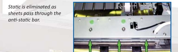
Air flows up from tray and floats paper stack. Stack positioning is much easier due to the reduction of friction between stack and tray.
